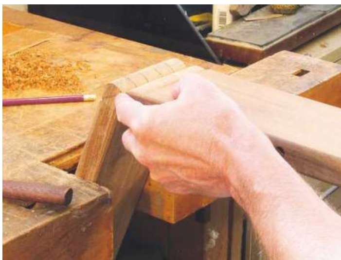
▲ Pic.8 Offer up both arms to check exactly which side of the line you want the saw cut to go
